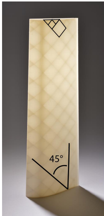
Figure 7: Outboard wing section, showing self-supporting angle and decreased cell size at top surface.
